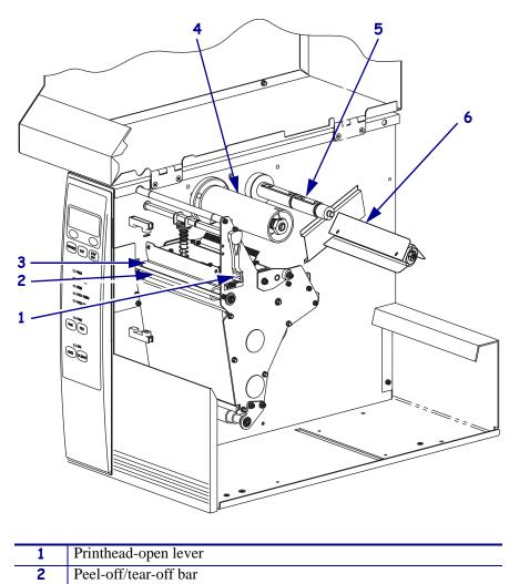
Figure 3 • Printer Components
